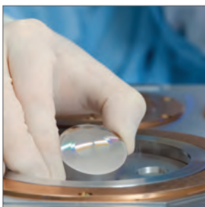
JPL researcher fabricating triple blaze gratings in the Microdevices Laboratory cleanroom.
