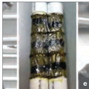
a-d The 340-GHz transceiver array has now enabled 8.3-Hz frame rate through-clothes standoff radar imaging for personnel screening security applications. Here are four frames of a movie including the real-time overlay of 340-GHz radar imagery of a fake pipe bomb (e) hidden underneath a heavy leather jacket. f Front-end of a 340-GHz imaging radar, showing a linear array of four submillimeter-wave transceivers based on MDL-fabricated Schottky diodes and a compact stack of MDL-fabricated micromachined silicon waveguide. g Portable imaging radar system.
