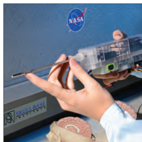
Laboratory prototype of MARVEL, one of the world's smallest, steerable 3D cameras.
