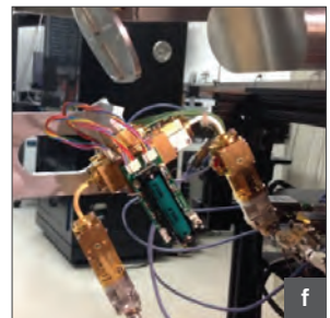
a-d The 340-GHz transceiver array has now enabled 8.3-Hz frame rate through-clothes standoff radar imaging for personnel screening security applications. Here are four frames of a movie including the real-time overlay of 340-GHz radar imagery of a fake pipe bomb (e) hidden underneath a heavy leather jacket. f Front-end of a 340-GHz imaging radar, showing a linear array of four submillimeter-wave transceivers based on MDL-fabricated Schottky diodes and a compact stack of MDL-fabricated micromachined silicon waveguide. g Portable imaging radar system.
