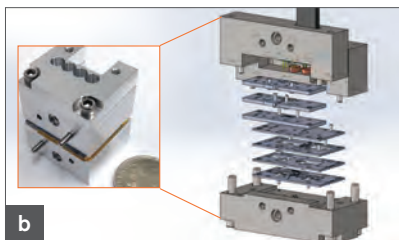
a. 550-GHz, dual-polarized sideband-separated receiver with silicon micromachined waveguide packaging. Silicon micromachined waveguide components are vertically stacked to form the highly integrated receiver front-end. b. MDL has built up advanced silicon micromachining capability that allows researchers to design and build submillimeter-wave components and instruments that are compact and well-suited for planetary missions. c, d. By utilizing advanced lithographic techniques available at MDL, JPL researchers have developed compact on-chip power combiners that allow manufacturing of high-power sources in the submillimeter-wave range, enabling atmospheric instruments with increased coverage.
